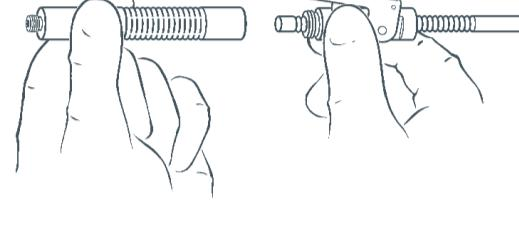
2. Remove the plunger by pulling the plunger through the "lever housing".
