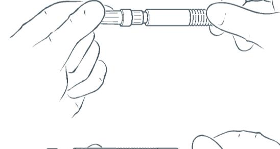
4. Insert a standard 1.8 ml. cartridge into the "barrel".
