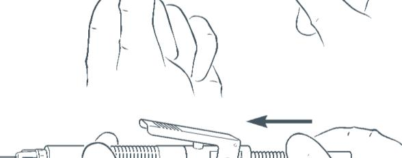
6. Insert the plunger into the "lever housing" and push it until contact is made with the cartridge.
