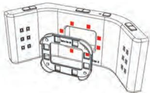
MDP with central LEDs at full power + polarizing filter, lateral LEDs off.
