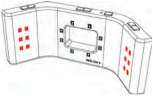
MDP with lateral LEDs at full power, central LEDs off.
