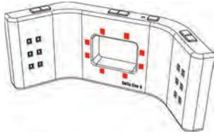
MDP with central LEDs at full power, lateral LEDs off.
