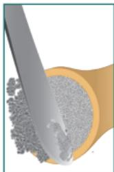
**1.** Use a cement spatula to remove excess powder. **DO NOT** use powder without leveling at the edge of the scoop.
