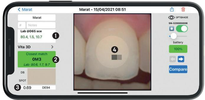
The information on the display of your phone is very clear and shows always the L\*a\*b\* coordinates of the measured tooth in comparison with the values of the closest recognized shade guide in the database.
