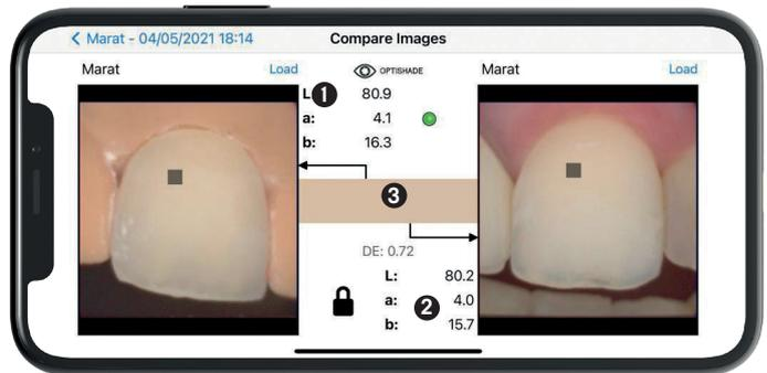
Compare function between the crown and the measurement of the natural tooth
